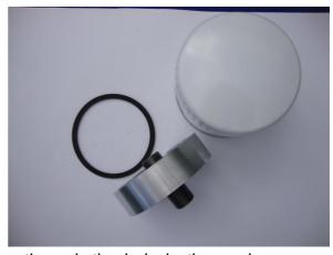
Ensure that the area around the oil filter housing is clean and remove the existing
